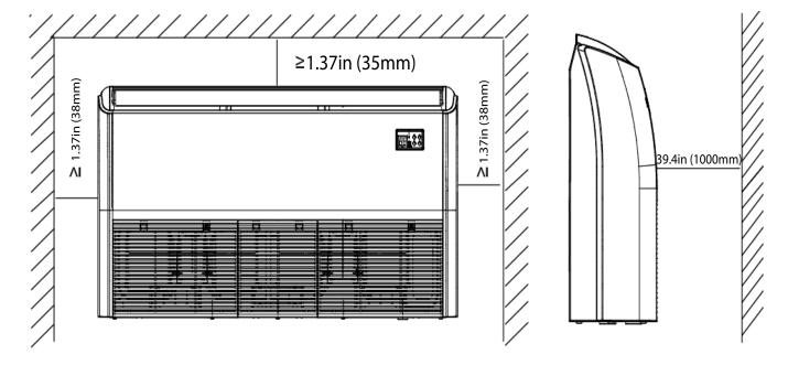
Fig. 7 — Clearance for 18K-24K
