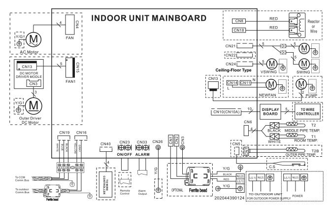
Fig. 14 — Wiring Diagram - Size 36K
