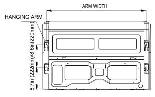
Fig. 5 — Indoor Unit Sizes 18K-58K
