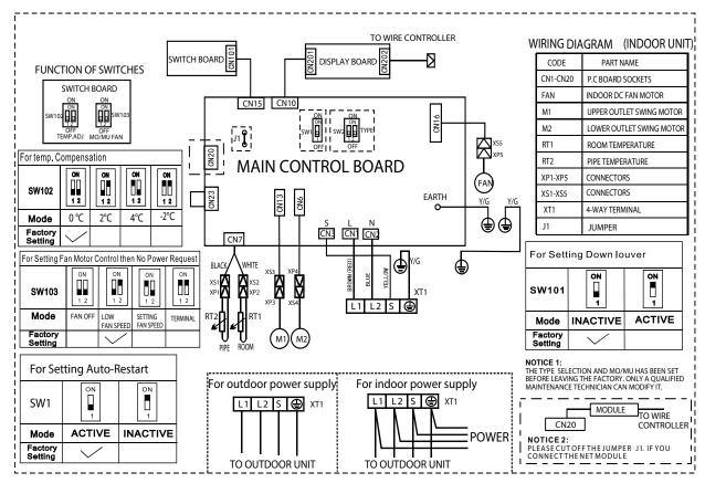
Fig. 12 — Wiring Diagram Size 12
