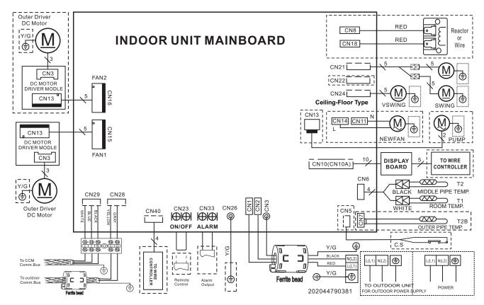
Fig. 15 — Wiring Diagram - Size 48K
