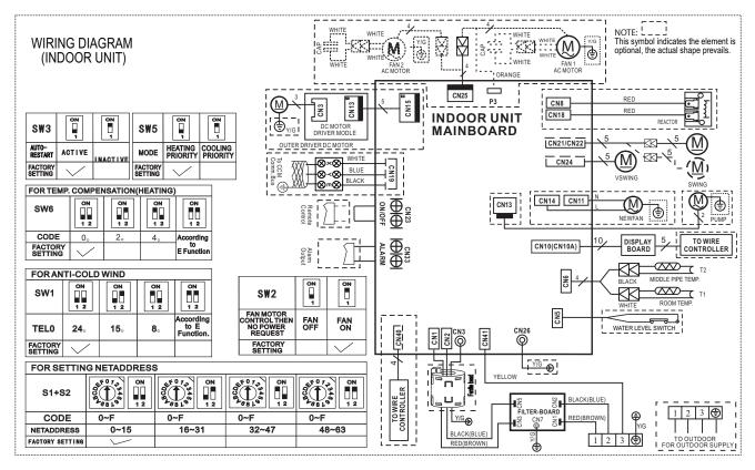
Fig. 13 — Wiring Diagram - Sizes 18K and 24K
