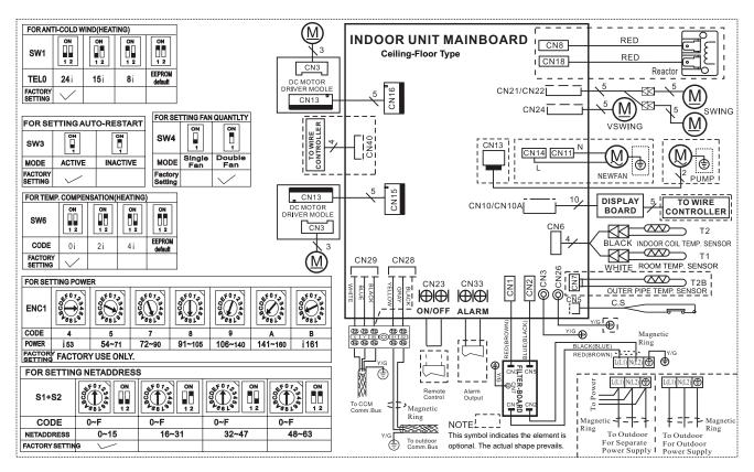
Fig. 16 — Wiring Diagram - Size 58K
