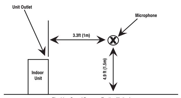
Fig. 11 — Sound Pressure Testing Method
